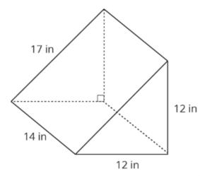
In general, we can find the volume of any prism by multiplying the area of its base times its height. For this prism, the area of the triangular base is  $72 \cdot 14$ , so the volume is  $72 \cdot 14$ , or 1,008 in<sup>3</sup>.
