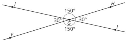
When two lines cross, they form two pairs of vertical angles across from one another. In the previous figure, angles JGF and HGI are vertical angles. So are angles JGH and FGJ. Vertical angles always have equal measures.
