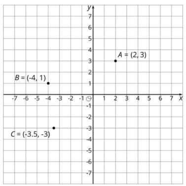
To find the distance between two points that share the same horizontal line or the same vertical lines, we can simply count the grid units between them. For example, if we plot the point (2, -4) on the grid above (try it!), we can tell that the point will be 7 units away from point A = (2, 3).
